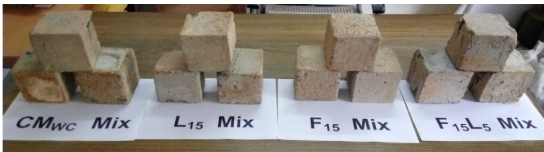
Fig.13 - Visual appearance of the specimens after 180 days immersion in HCl solution.
