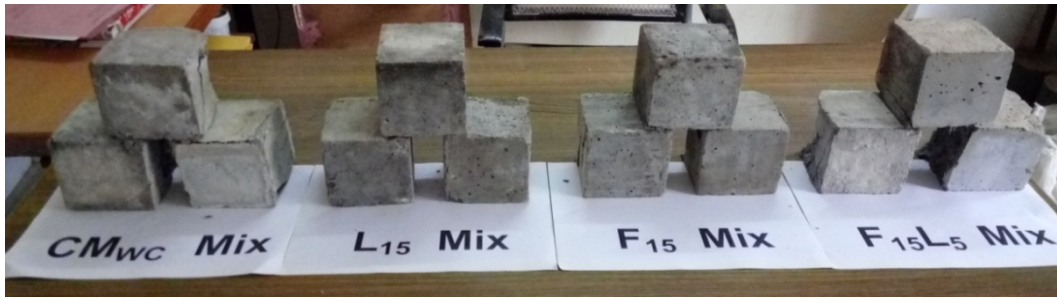
Fig.10 - Visual appearance of the specimens after 180 days immersion in MgSO 4 solution
