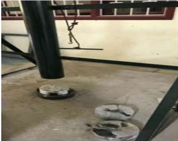
Fig. 1 - Drop weight impact test setup
