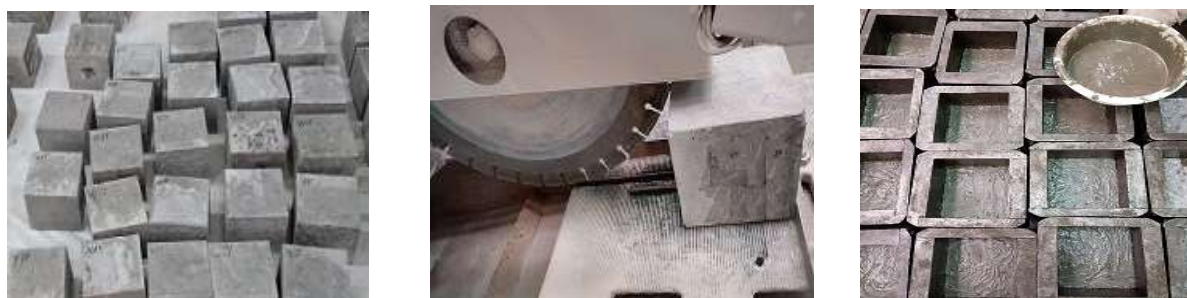
a) Substrate Concrete b) Cutting the substrate with saw c) Applying Grout over the substrate Fig. 1 - Stages of producing the samples required to measure the existing mortar-concrete adhesion
