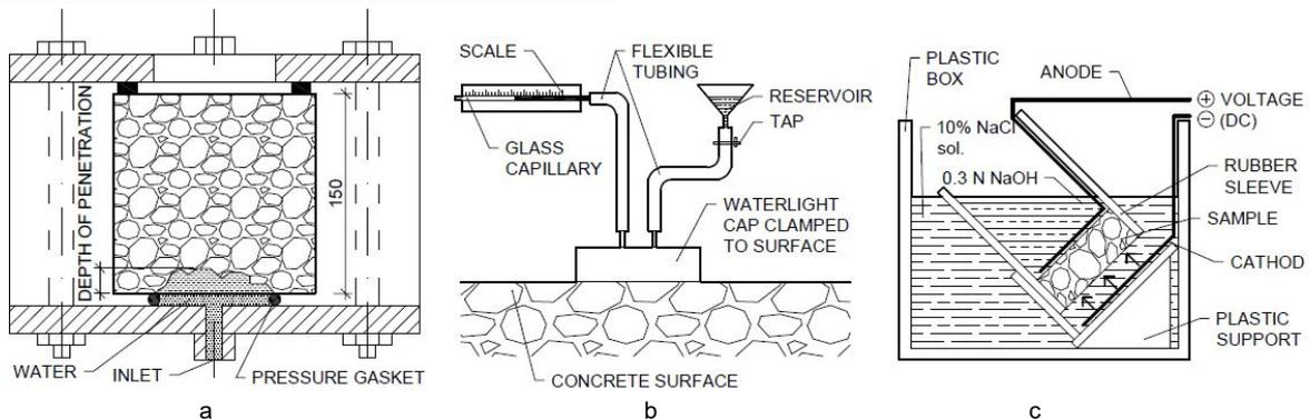
Fig. 1 - Illustration of the conducted permeability tests; a) water penetration test, b) ISAT, c) chloride migration test.
