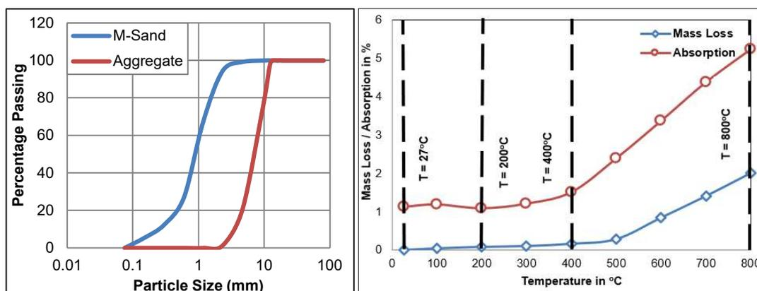
Fig. 1. a) Particle size distribution b) Physical properties of coarse aggregates subjected to elevated temperatures
