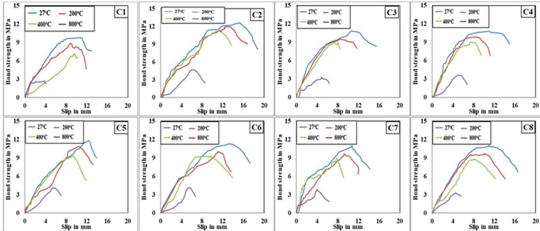
Fig. 8 - Bond-slip characteristics of the tested specimens
