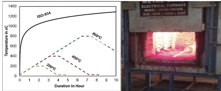
Fig. 2 - (a) Heat curve and ISO 834 curve (b) Specimen kept in Furnace
