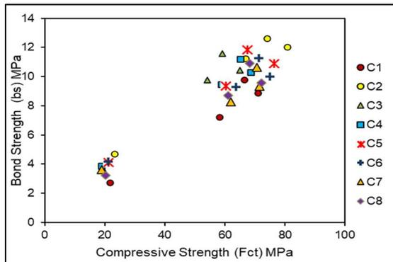
Fig.9 - Peak bond strength and compressive strength correlation graph
