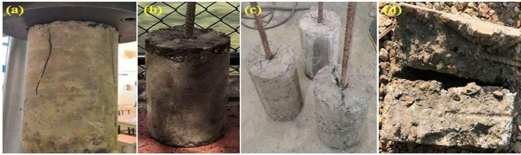
Fig. 7 - Visual observation of the exposed specimens (a) Development of cracks under testing, (b) spalling of concrete at corners, (c) crack width variation with and without fibres, (d) split specimens after testing.
