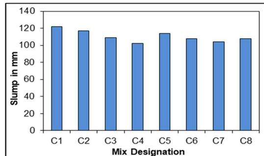
Fig. 3 - Slump cone results of the tested mixes
