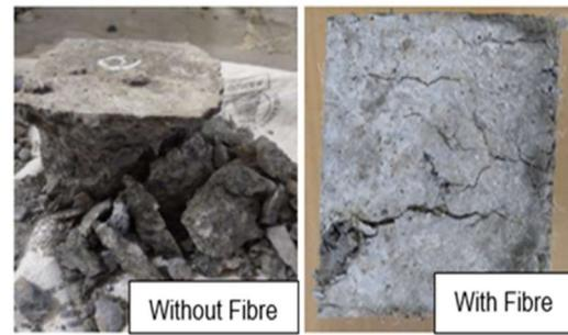
Fig. 5 - Failure pattern of 800°C exposed specimen
