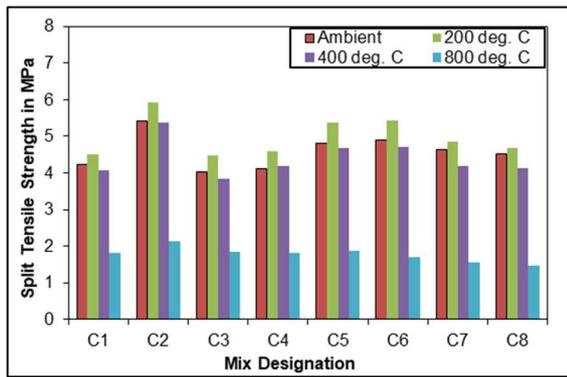
Fig. 6 - Split tensile strength results of the tested mixes at different temperature exposure
