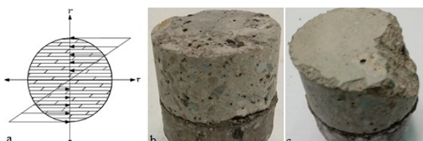
Fig. 2 - Creation of Stress and Failure in the "Twist-off" Method; a) Maximum shear stress, b) failure at common boundary, c) composite failure.
