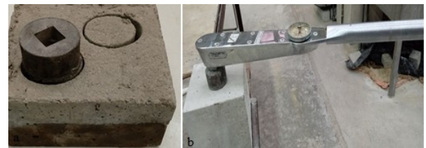
Fig. 1 - Performing "Twist-off" Test; a) The determination of shear bond strength, b) the evaluation of repair mortar compressive strength.
