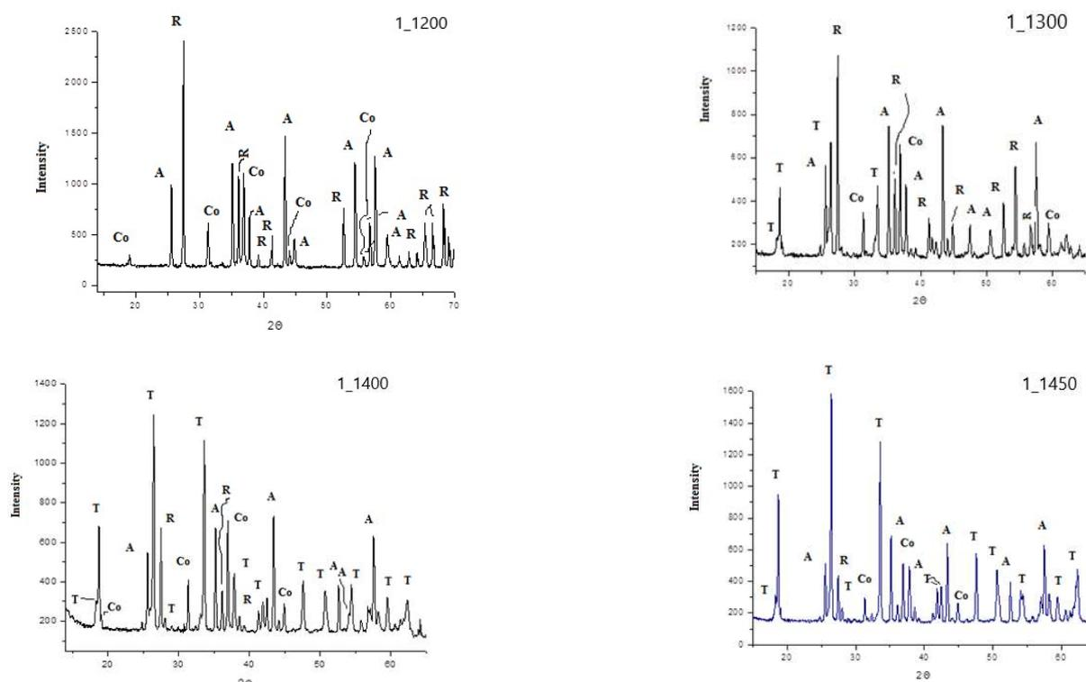
Fig. 1 - X-ray patterns of sample 1 depending on the combustion temperature; T - tialite; A - corindon; R - rutil; Co-ss (MgAl<sub>2</sub>O<sub>4</sub>-CoAl<sub>2</sub>O<sub>4</sub>)
