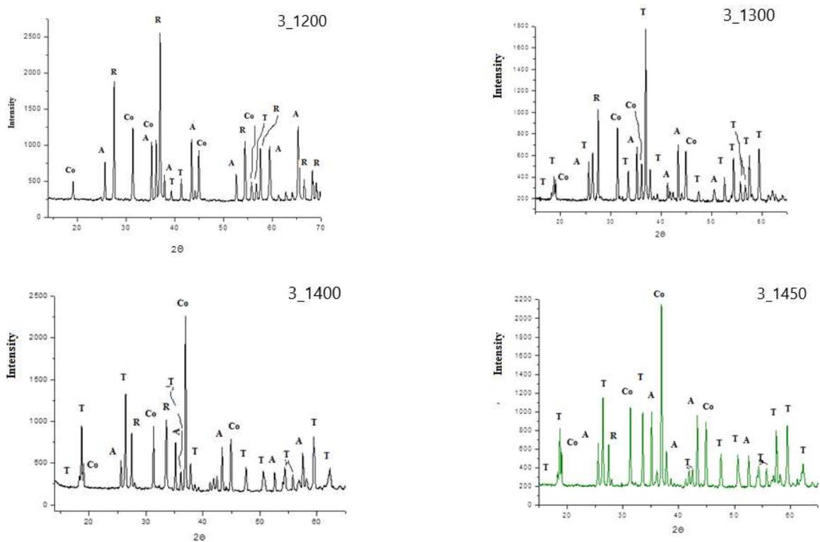
Fig. 3 - X-ray patterns of sample 3 depending on the combustion temperature; T-tialite; A-corundum; R-rutile; Co-ss ( $MgAl_2O_4-CoAl_2O_4$ )
