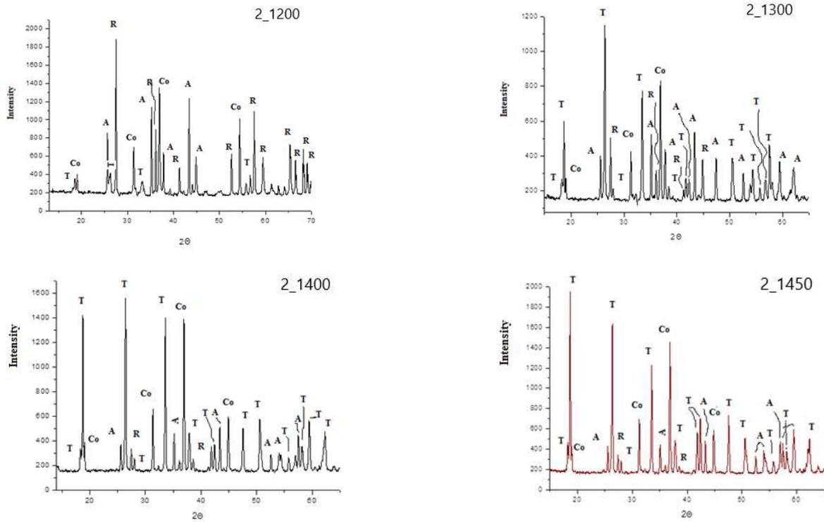
Fig. 2 - X-ray patterns of sample 2 depending on the combustion temperature; T-tialite; A-corundum; R-rutile; Co-ss ( $MgAl_2O_4-CoAl_2O_4$ )
