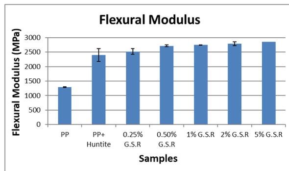
Fig. 5. Flexural modulus of a) glass fibers, b) glass spheres reinforced composites.
