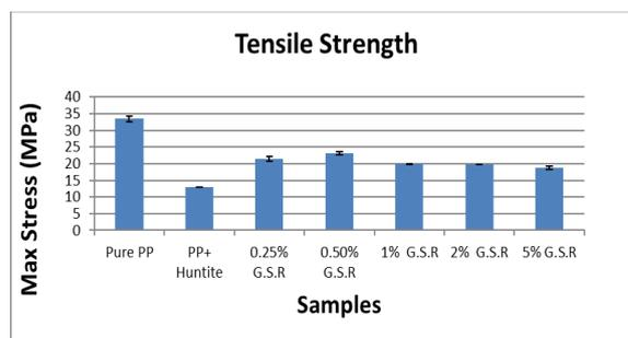
Fig. 3 - Tensile strength of a) Glass fibers, b) Glass spheres reinforced composites.
