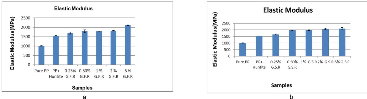
Fig. 2 - Elastic modulus of a) Glass fibers and b) Glass spheres reinforced composites.
