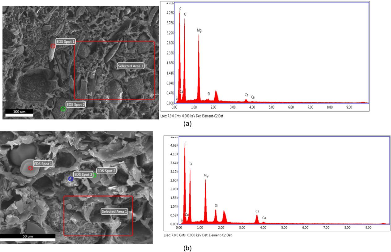
Fig. 1 - EDS analysis of a) 5 % glass fibers and b) 5% glass spheres reinforced composites.
