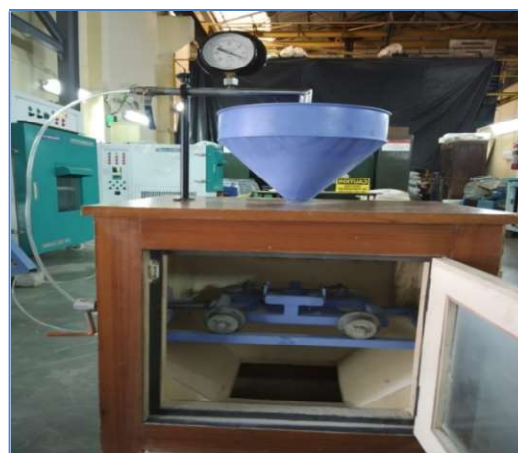
Fig. 2 - Abrasion of concrete (IS 9284) test set up.
