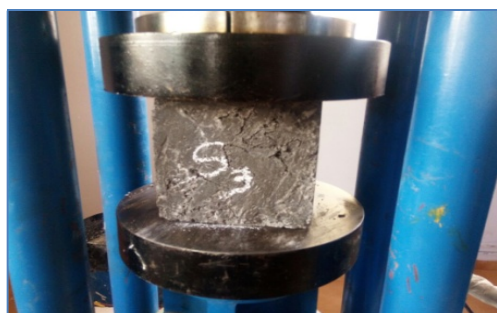
Fig. 1 - Compression testing on concrete specimen.
