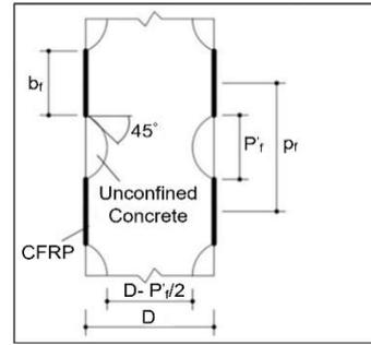
Fig. 6 - Elevation view of concrete member confined with FRP strips [5]
