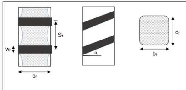
Fig. 3 - Illustration of the dimensional variables used in strengthening calculations for CFRP strips. [6].
