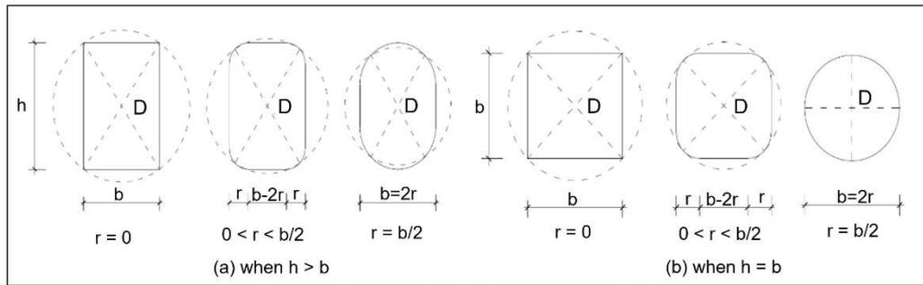
Fig. 8 - Diameter of the equivalent concrete cylinder [3].
