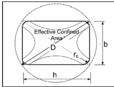
Fig. 2 - Equivalent circular cross section. [6].
