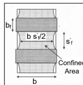
Fig. 5 - Confinement with FRP strips [7].
