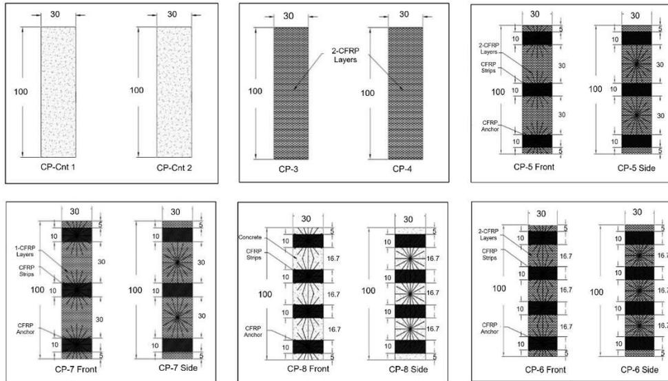
Fig. 1 - Test specimen's details. (dimensions in cm)
