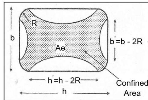
Fig. 4 - Effectively confined concrete in rectangular cross section [7].
