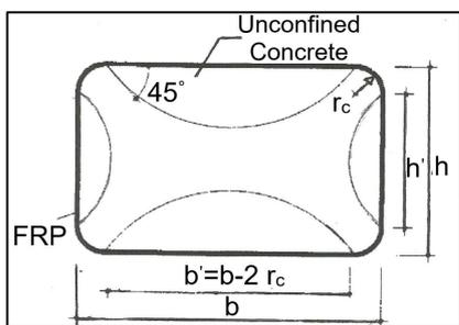
Fig. 7 - Confinement of rectangular sections
