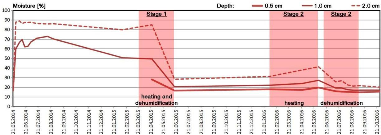
Fig. 9 - Moisture of the CBPB at various depths during the monitoring of the building.
