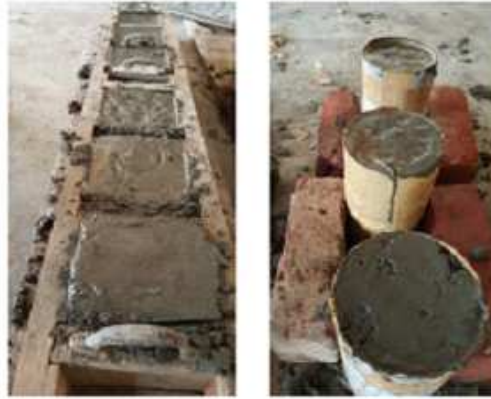
Fig. 2 - Casting of Cubes and Cylindrical specimens in the wooden mould.
