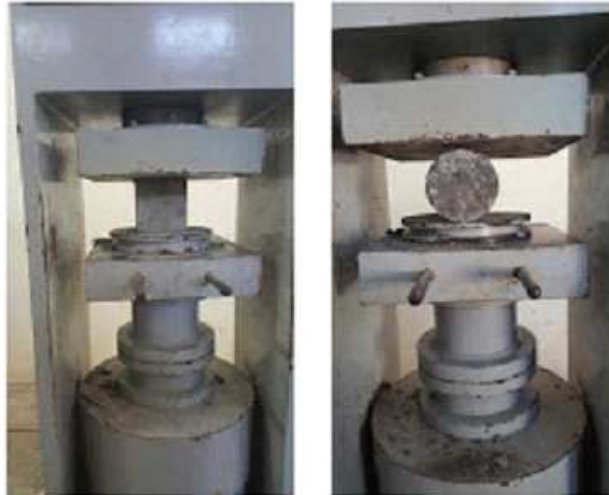
Fig. 3 - Testing of Cubes and Cylindrical specimens in DCTM.
