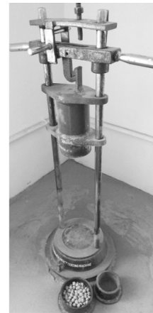
Fig. 2 - Aggregate impact test apparatus.
