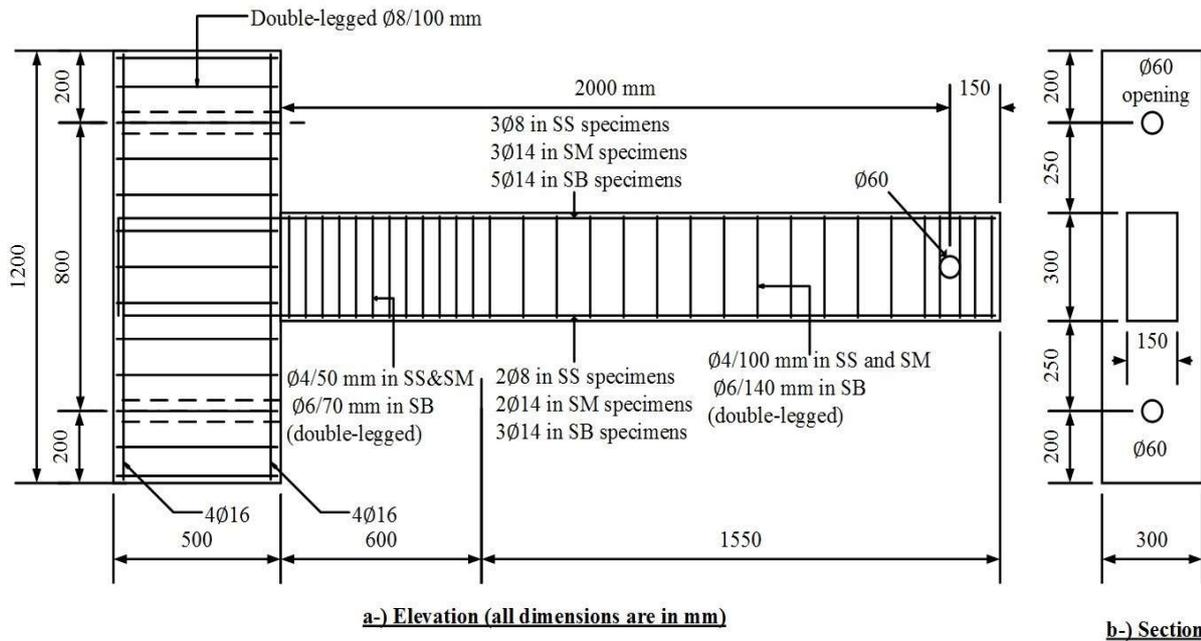
Fig. 1 - Test specimen details
