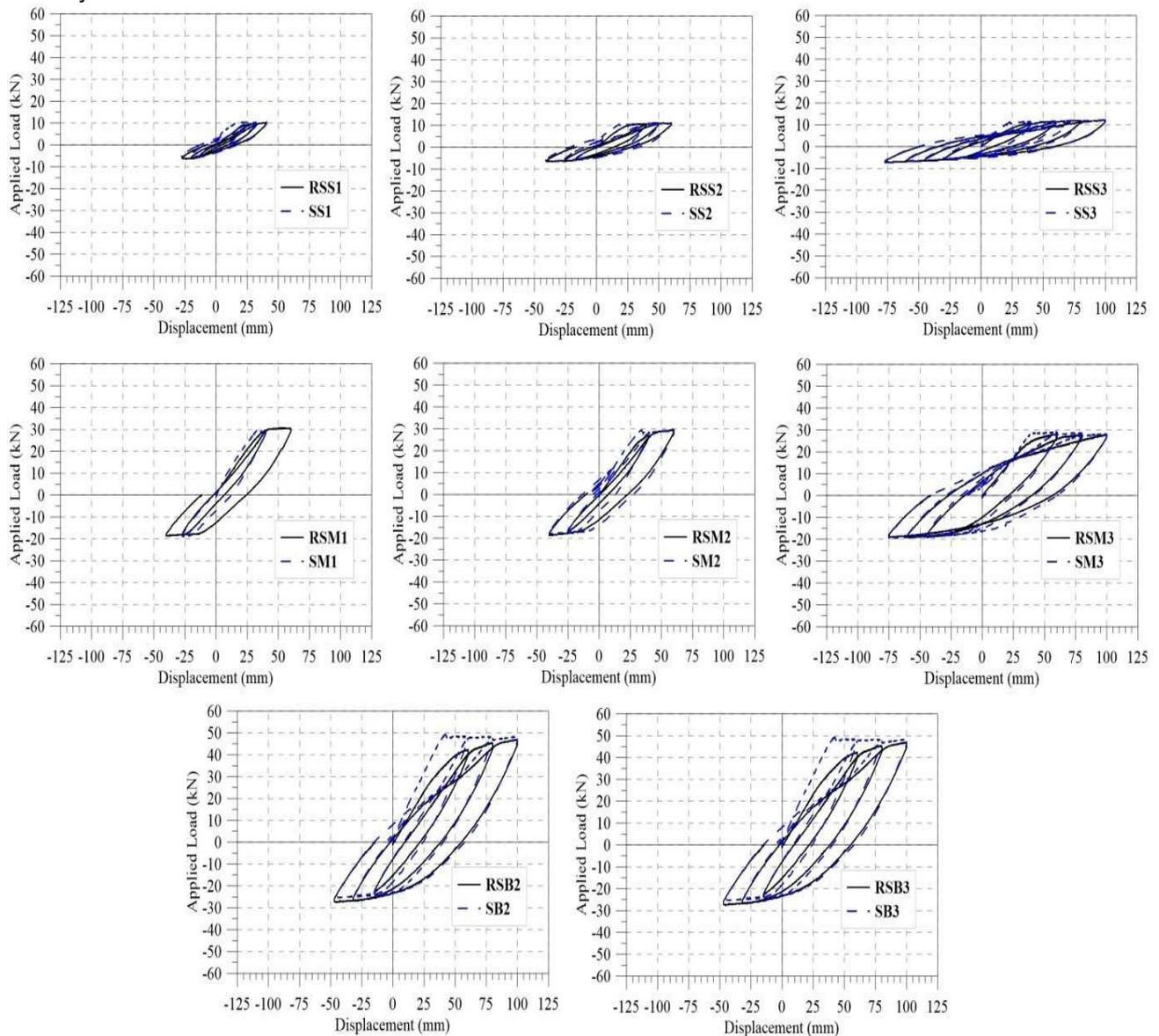
Fig. 10 - Load-deflection curves of specimens
