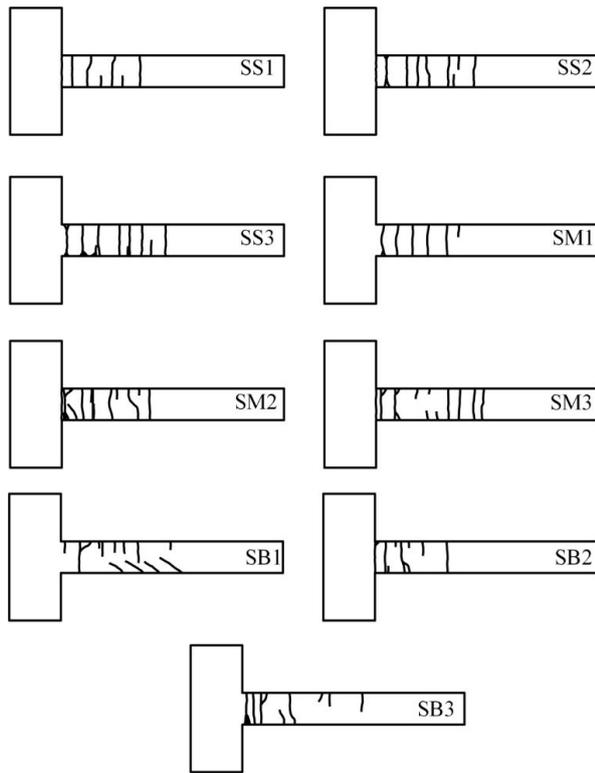
Fig. 7 - Final crack patterns of the virgin specimens
