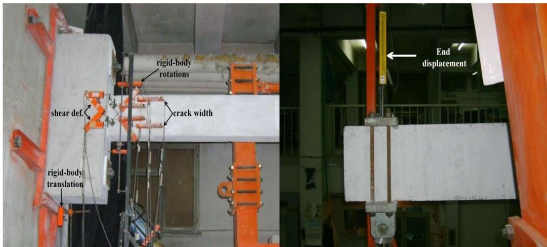
Fig. 6 - LVDT's in the tests
