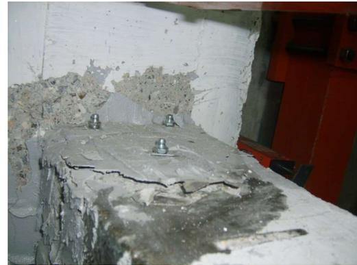
Fig. 9 - Disintegration of the epoxy layer and nozzles (ports)
