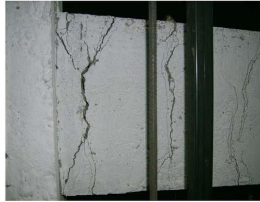
Fig. 8 - Extensive cracking in specimen with medium and high reinforcement ratio
