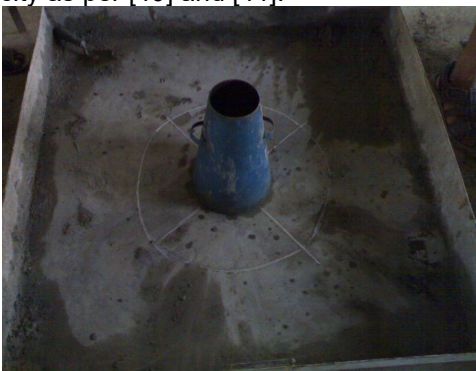
Fig. 3 - Slump and T_{50\text{cm}} slump flow test set up
