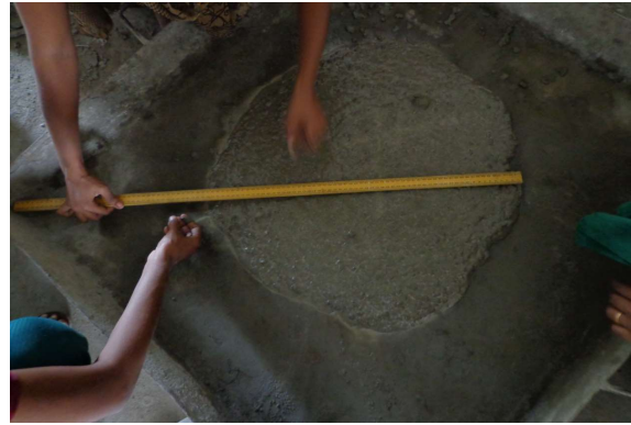
Fig. 4 - Slump flow measurement
