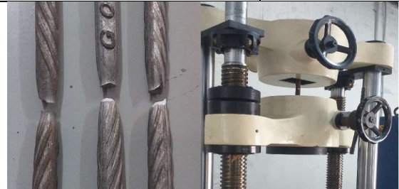
Fig. 2 - Tensile strength test on deformed bar
