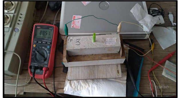
Fig. 4- Current passage measurement in mortars.
