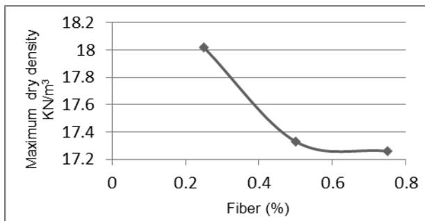
Fig. 11 - The changes diagram of fibre% and maximum dry density (in a mix composition of 30% microsilica + 6 % cement).
