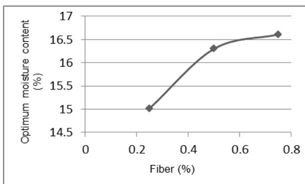
Fig. 12 - The changes diagram of Fibre% and optimum moisture content (in a mix composition of 30% microsilica + 6 % cement).
