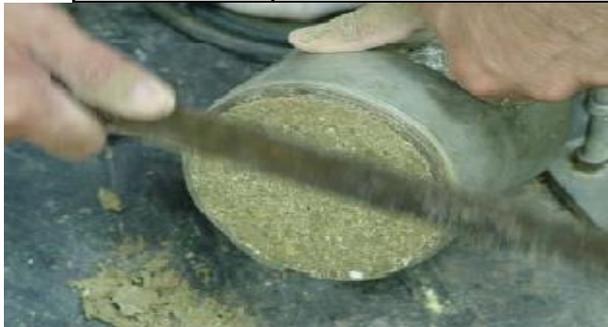
Fig. 7 - Density testing based on ASTM D1557-70 standard
