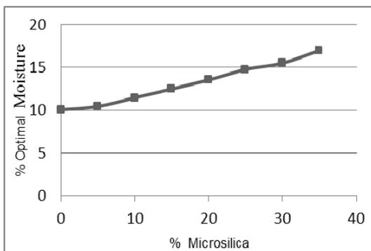
Fig. 8 - Microsilica amount and optimal moisture graph.
