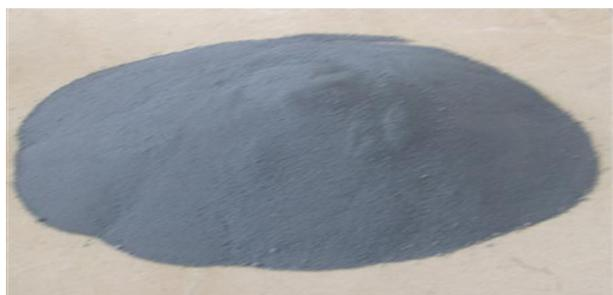
Fig. 4 - Microsilica used in specimens
