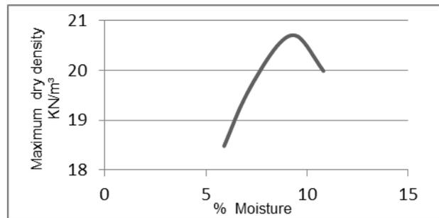
Fig. 3 - Modified density testing Graph.
