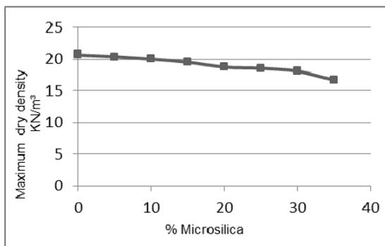
Fig. 9 - Microsilica amount and maximum dry density graph.
