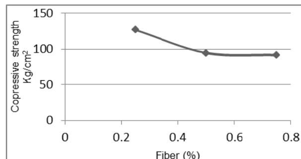
Fig. 13 - Changes graph of compressive strength-fibres percentage.
