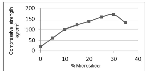
Fig. 10 - Microsilica amount and compressive strength graph.
