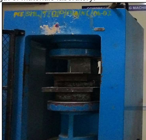
Fig. 8 - Typical testing method for Compressive strength on concrete cubes
