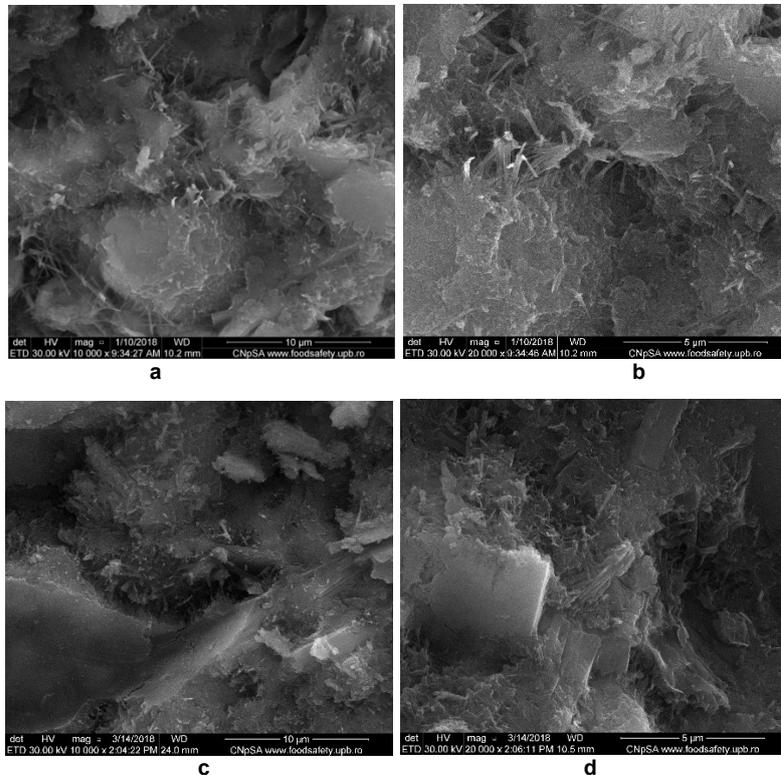
Fig. 4 – Scanning electron microscopy images for E hardened for 28 days (a, b) and 90 days (c, d)
