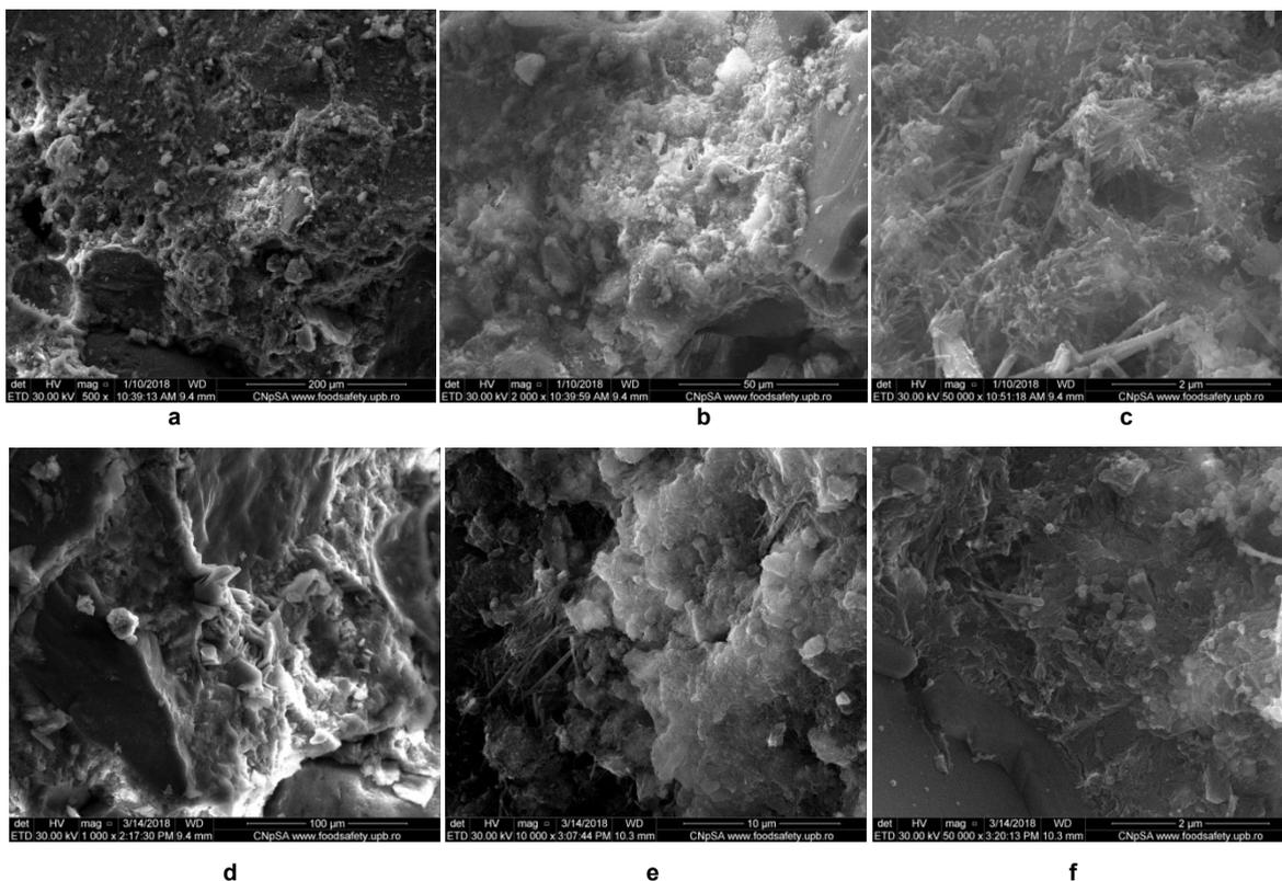
Fig. 5 – Scanning electron microscopy images for BT15 hardened for 28 days (a, b, c) and 90 days (d, e, f).
