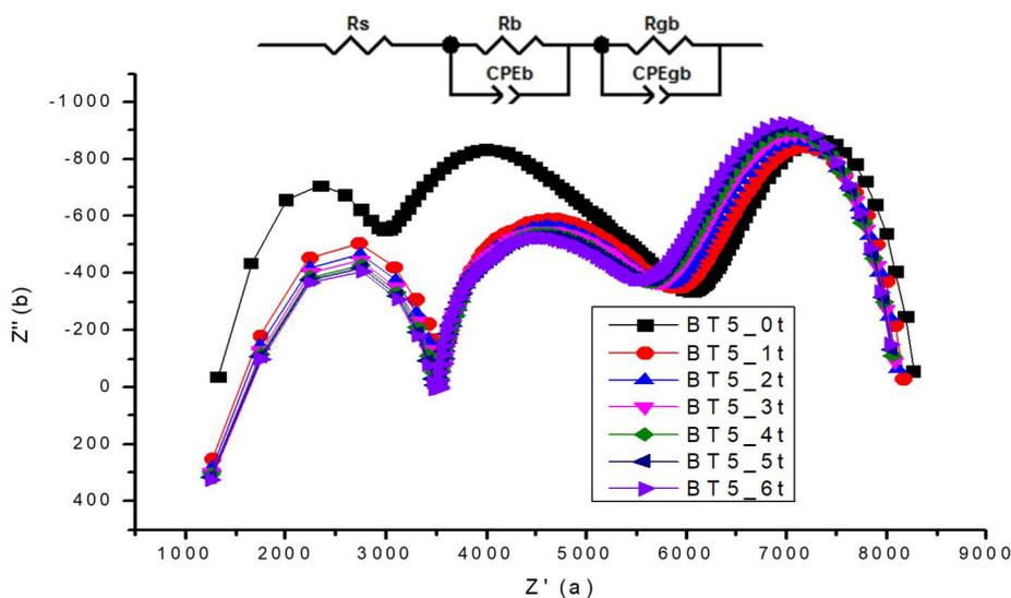
Fig. 6 – Impedance plot for BT5 hardened for 28 days with different loading effort and equivalent circuit (detail above).
