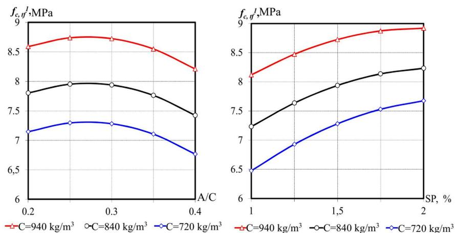
Fig. 2 - Effect of technological factors on flexural strength of RPC at 1 day
