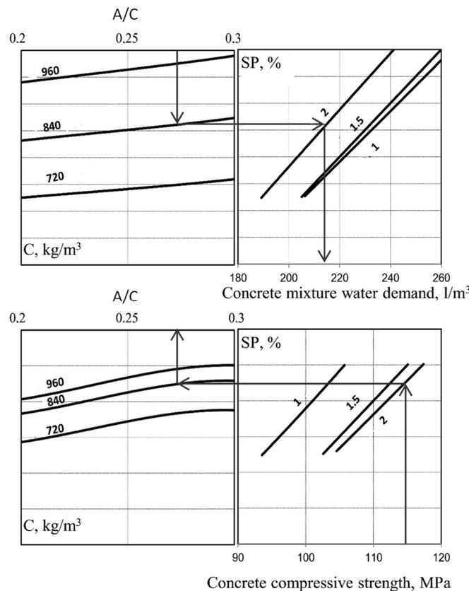
Fig. 8 - Nomograms of water demand and compressive strength of RPC made using activated fly ash
