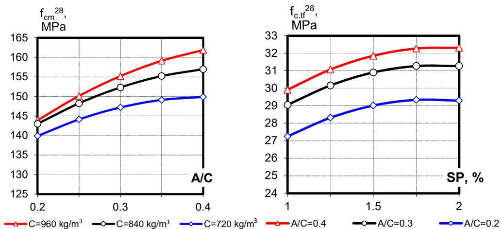
Fig. 7 - The influence of the studied factors on the flexural strength ( $f_{c,tf}$ , MPa) and compressive strength ( $f_{cm}$ , MPa) of RPC with microsilica at the 28 days.
