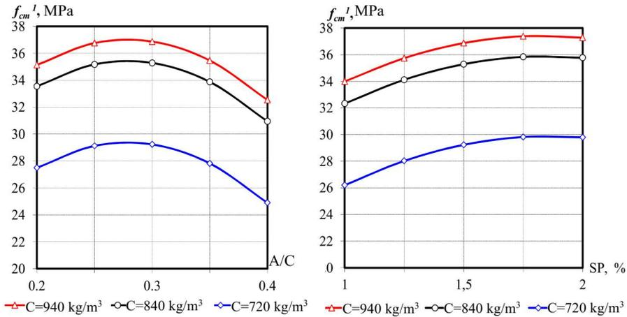
Fig. 3 - Effect of technological factors on compressive strength of RPC using fly ash at 1 day
