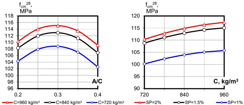
Fig. 5 - Effect of technological factors on compressive strength of RPC produced using fly ash at 28 days
