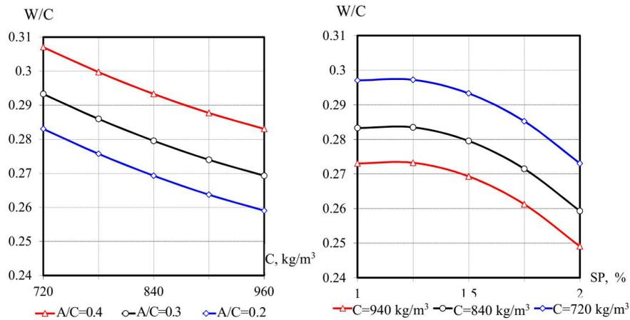
Fig. 1 - Effect of technological factors on water-cement ratio of RPC produced using fly ash
