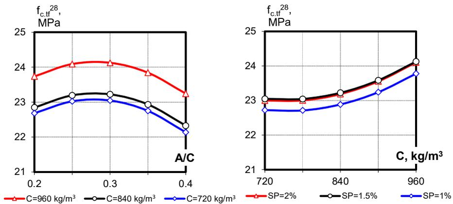
Fig. 4 - Effect of technological factors on flexural strength of RPC produced using fly ash at 28 days
