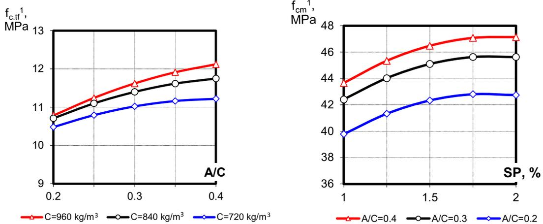
Fig. 6 - The influence of the studied factors on the flexural strength ( $f_{c,tf}$ , MPa) and compressive strength ( $f_{cm}$ , MPa) of RPC with microsilica at the 1 day.
