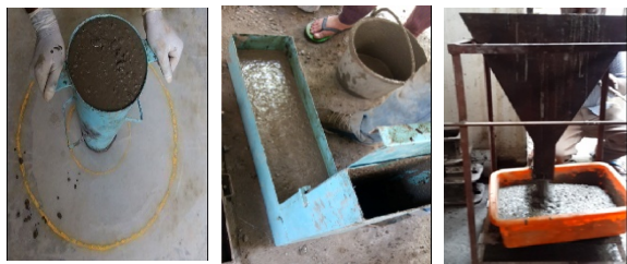
(a) Slump flow and T_{50} cm flow (b) L-Box (c) V-Funnel Fig. 1 - Some of the fresh Properties tests of SCC.
