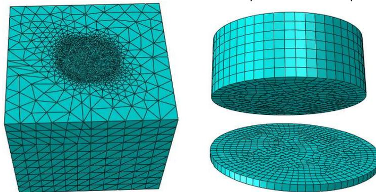
Fig. 15 - The meshing of the model.
