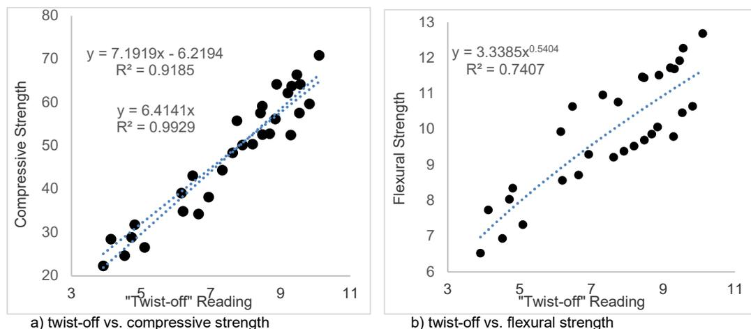
Fig. 8 - The correlation between the twist-off results and the mechanical properties of the fiber reinforced mortars.
