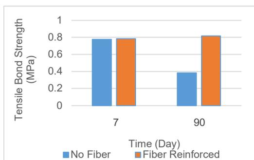
Fig. 12 - Tensile bond strength results of the "Pull-off" Test.
