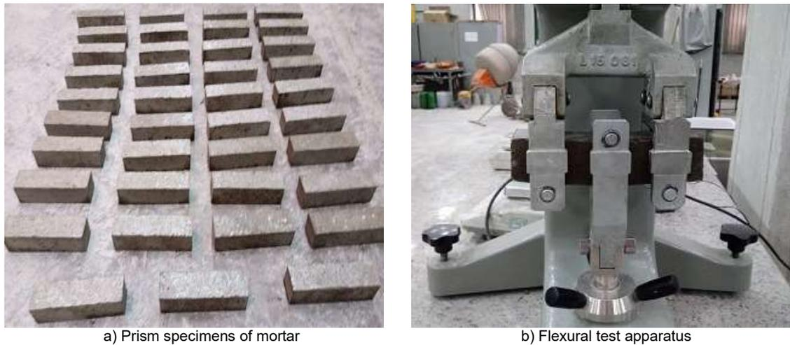
a) Prism specimens of mortar b) Flexural test apparatus
