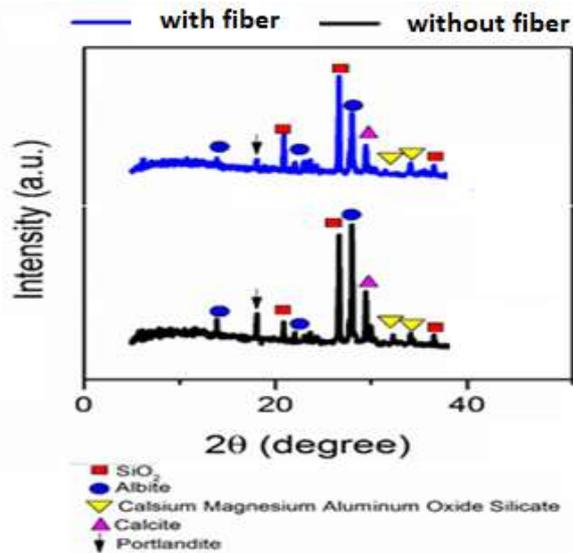
Fig. 6 - X-ray diffraction pattern for fiber-reinforced mortar.
