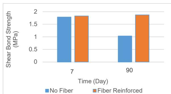
Fig. 11 - Shear bond strength results of the "Twist-off" Test.
