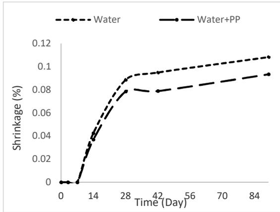
Fig. 14 - Dry shrinkage of mortars.
