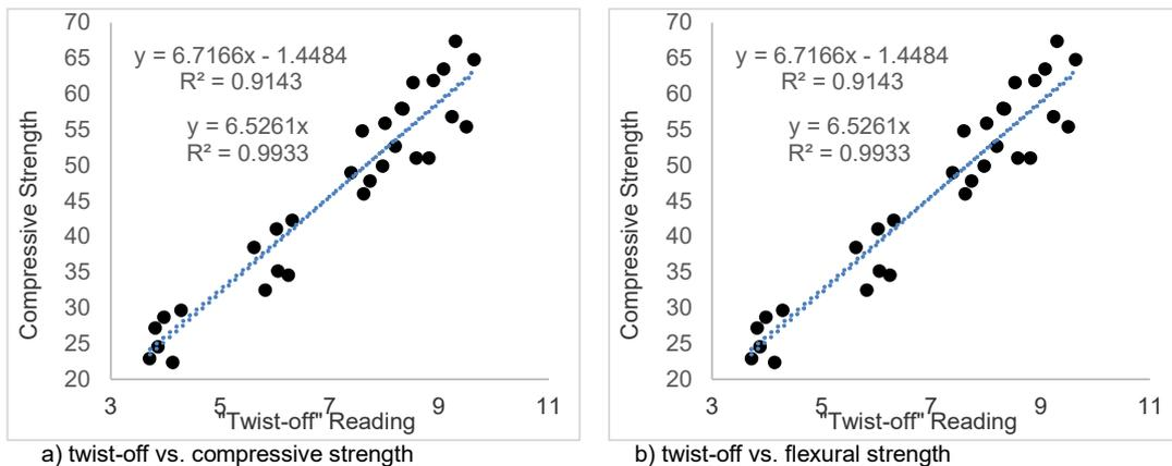
Fig. 7 - The correlation between the twist-off results and mechanical properties of the cement mortars without fibers.
