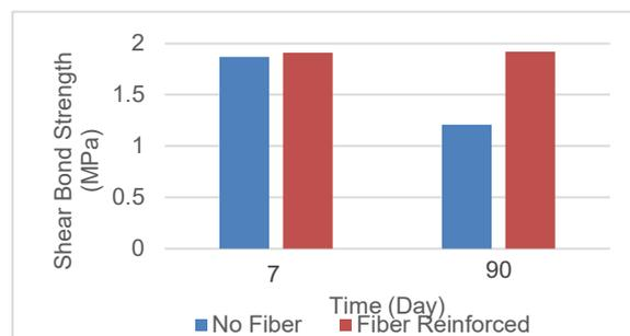
Fig. 13 - Shear bond strength results of the "Push-out" Test.
