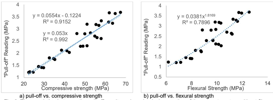
Fig. 9. The correlation between the pull-off results and mechanical properties of the cement mortars without fibers.
