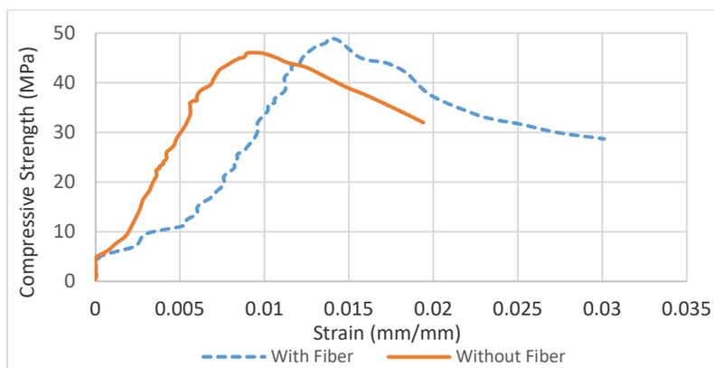
Fig. 4 - The effects of fibers on the compressive behavior of the mortars.
