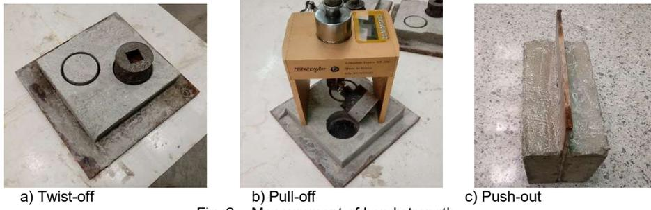
a) Twist-off b) Pull-off c) Push-out
