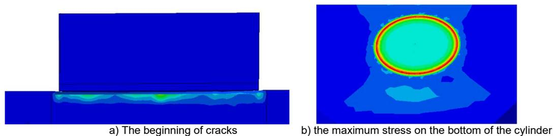
Fig. 17 - The pull-off test.
