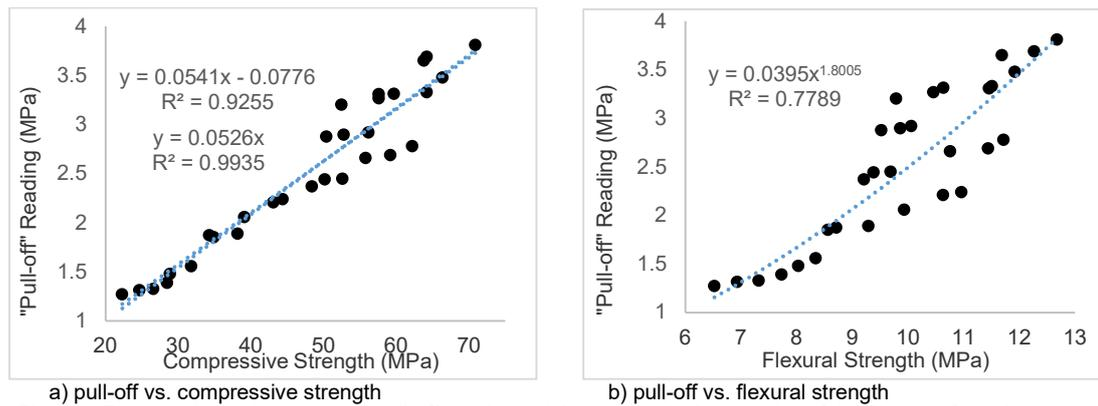
Fig. 10 - The correlation between the pull-off results and the mechanical properties of the fiber reinforced mortars.
