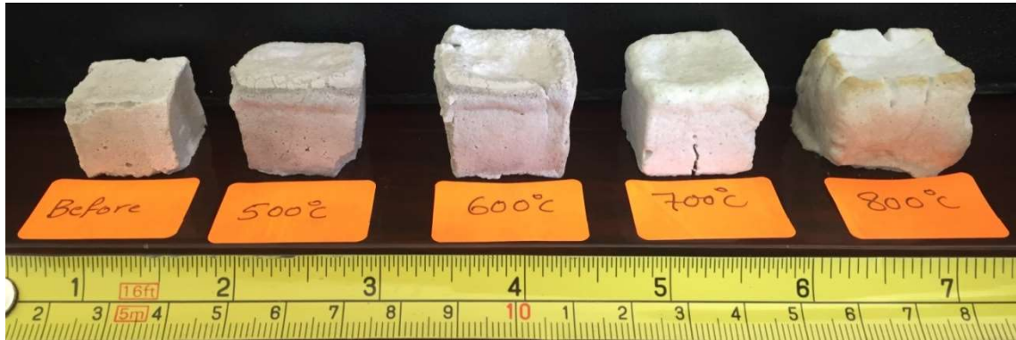
Fig.4 - MGG-N5 paste specimen's before and after thermal treatment at 500, 600, 700 and 800 °C /1h.
