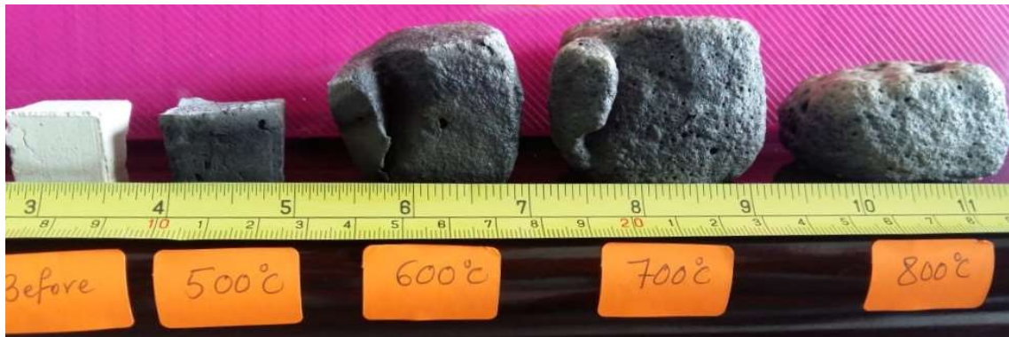
Fig.5 - MGIG-N5 paste specimen's before and after thermal treatment at 500, 600, 700 and 800°C /1h.
