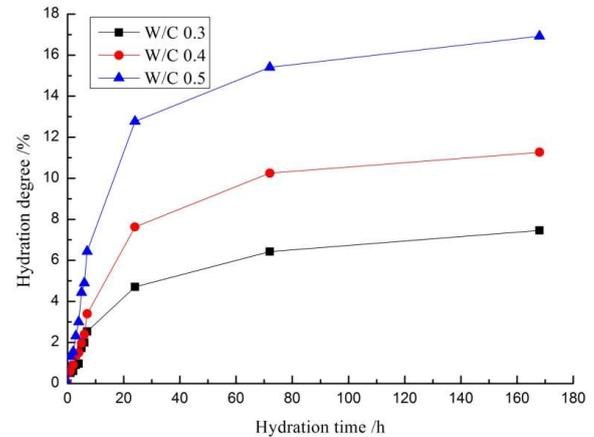
Fig. 6 - Hydration degree of cement pastes with W/C ratios of 0.3, 0.4 and 0.5
