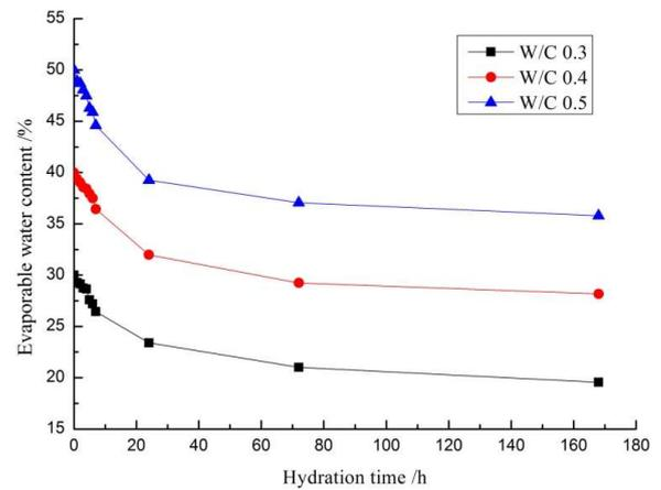
Fig. 5 - The evaporable water contents of cement pastes during hydration
