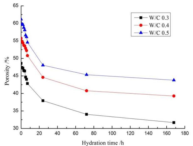
Fig. 8 - The porosity of cement pastes during hydration
