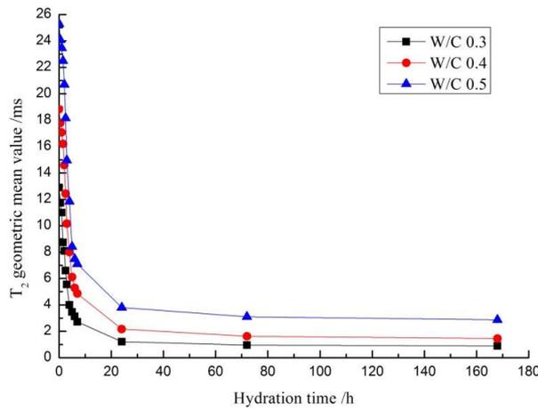
Fig. 4 - Changes of T<sub>2</sub> geometric mean value during hydration
