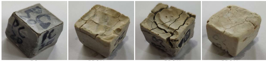
Fig. 6- Appearances of cement paste samples pre-cured at 20 °C and then eroded by sulfate solution for 180 d
