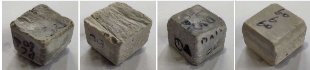
Fig. 7- Appearances of cement paste samples pre-cured at 60 °C and then eroded by sulfate solution for 180 d
