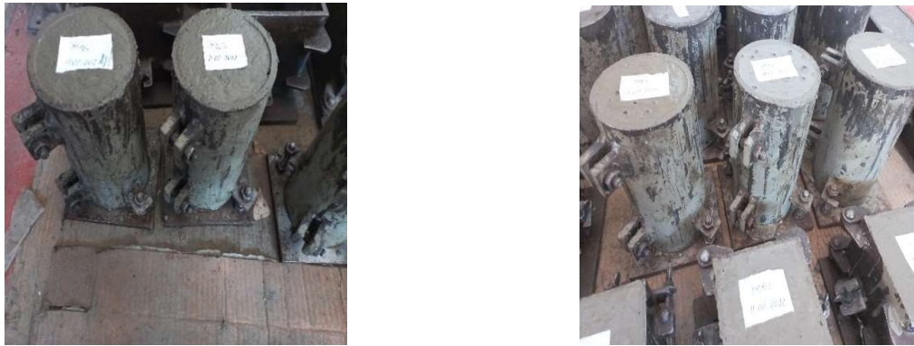
Fig. 2 - Making the test specimens / Realizarea epruvetelor
