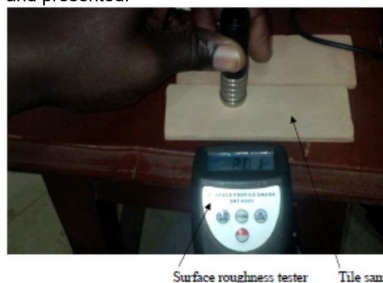
Fig. 1 - Digital surface roughness gauge used for the experiment
