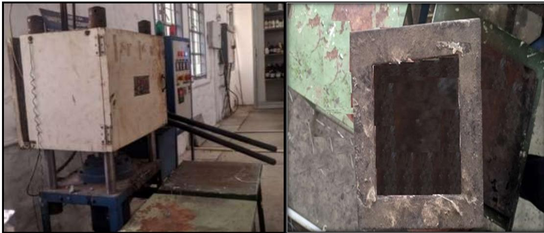
Fig. 1 - Compression molding Machine and mold for fabrication
