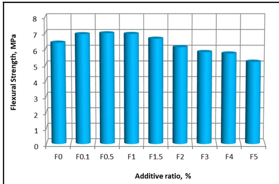
Fig. 4 - Flexural strength of the cement mortar containing Fe<sub>3</sub>O<sub>4</sub>/humic acid.
