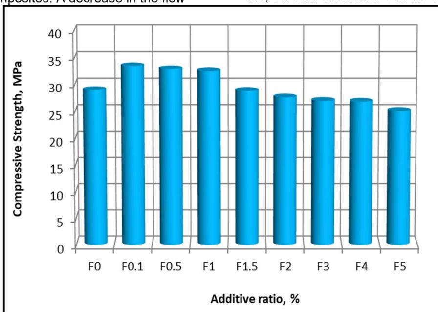
Fig. 5 - Compressive strength of the cement mortar containing  $Fe_3O_4$ /humic acid.
