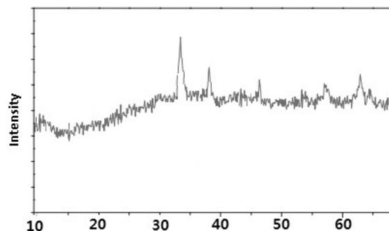
Fig. 2 - XRD pattern Fe<sub>3</sub>O<sub>4</sub>/humic acid magnetic nanocomposites.
