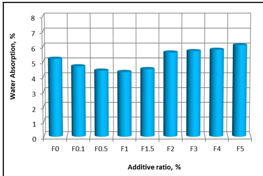
Fig. 6 - Water absorption of the cement mortar containing  $\text{Fe}_3\text{O}_4$ /humic acid.
