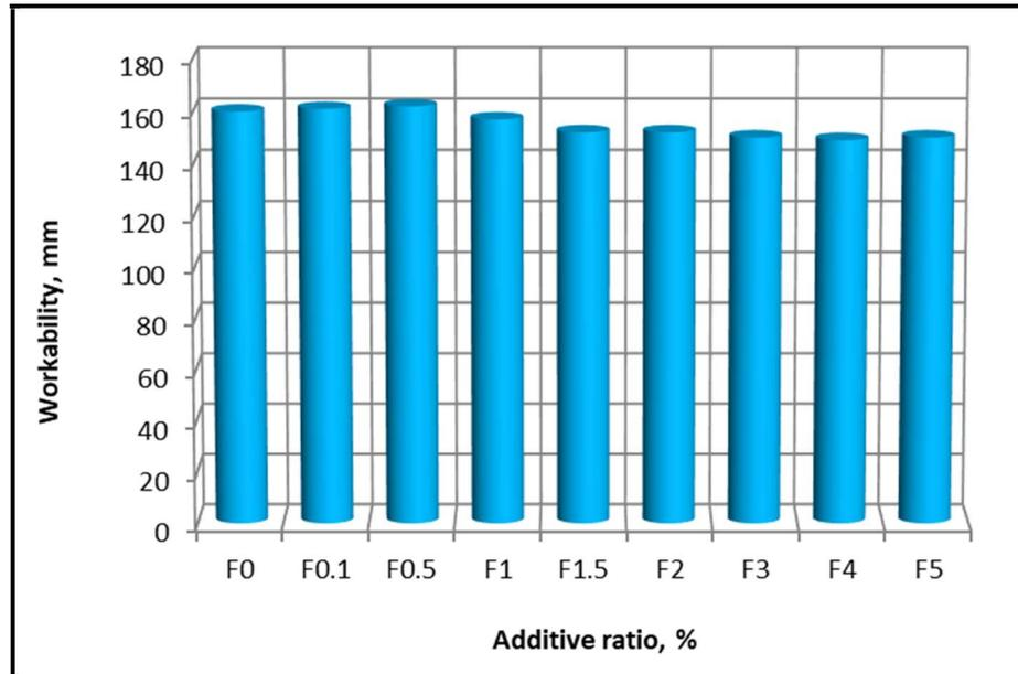
Fig. 3 - Workability of the fresh mortars.
