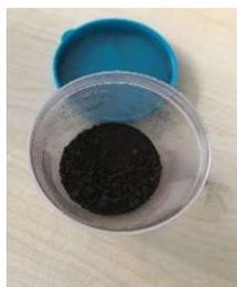
Fig. 1 - Fe<sub>3</sub>O<sub>4</sub>/humic acid nanoparticles.
