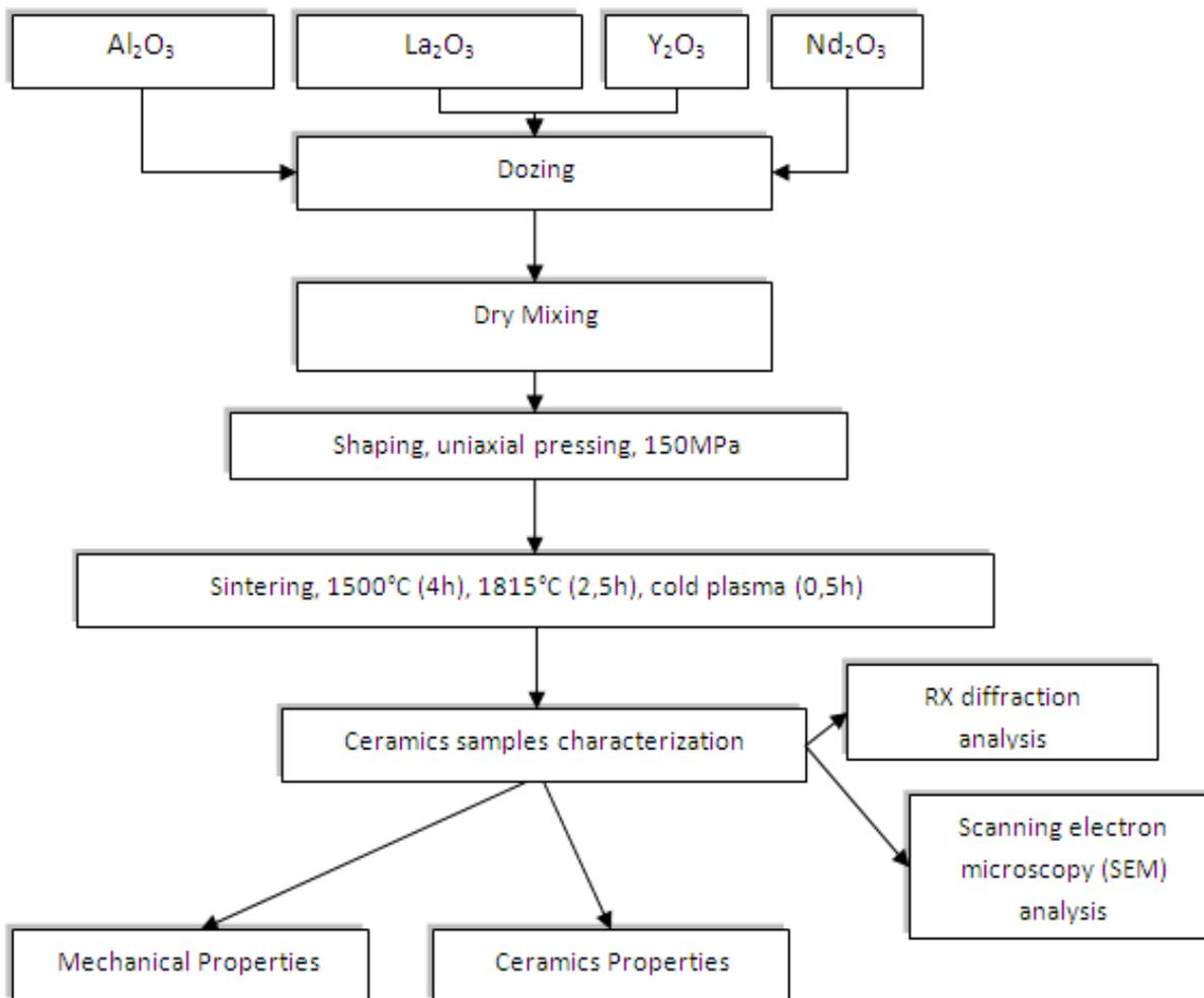
Fig. 1- Processing flow chart / *Fluxul tehnologic.*
