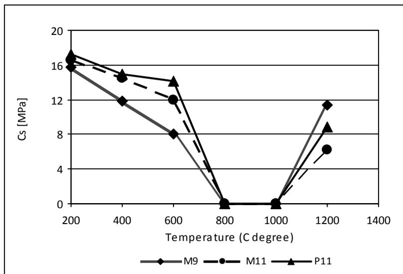
Fig.1 - Compressive strengths of the binding samples, heat treated at 200- 1200 Celsius degrees / *Rezistența la compresiune a probelor liante, tratate termic la 200-1200°C.*
