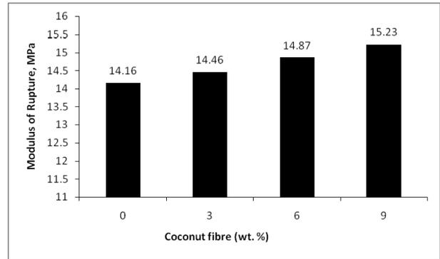
Fig. 7 - Modulus of rupture of composites for 28 days curing /
