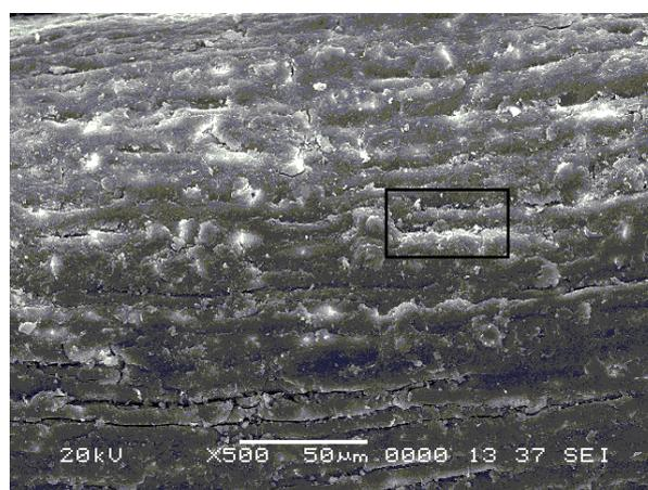
Fig. 3 - SEM image of a coconut fibre at 500x magnification. Imagine SEM a unei fibre de cocos la o mărime de 500x.
