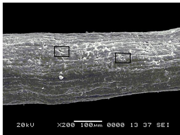
Fig. 2 - SEM image of a coconut fibre at 200x magnification. Imagine SEM a unei fibre de cocos la o mărime de 200x.
