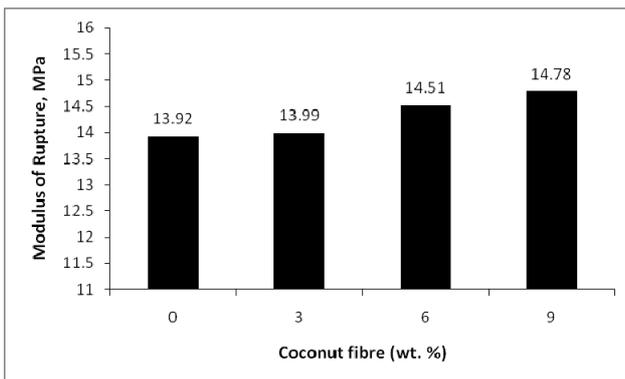
Fig. 6 - Modulus of rupture of composites for 14 days curing.
