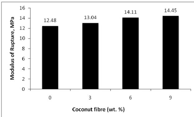
Fig. 5 - Modulus of rupture of composites for 7 days curing .
