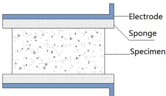
Fig. 2- Connection graph of electrode and specimens for electrical resistivity measurement.
