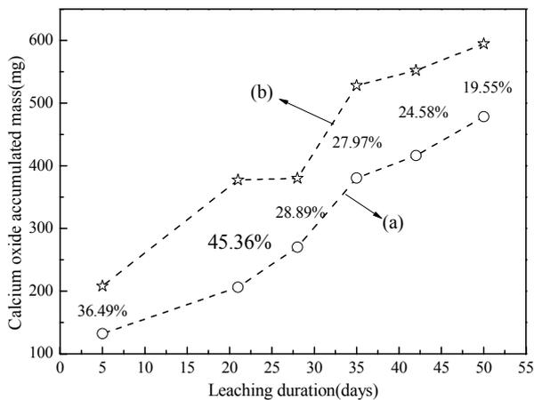
Fig. 4 - Calcium oxide accumulated mass (a) single test and (b) coupled test.
