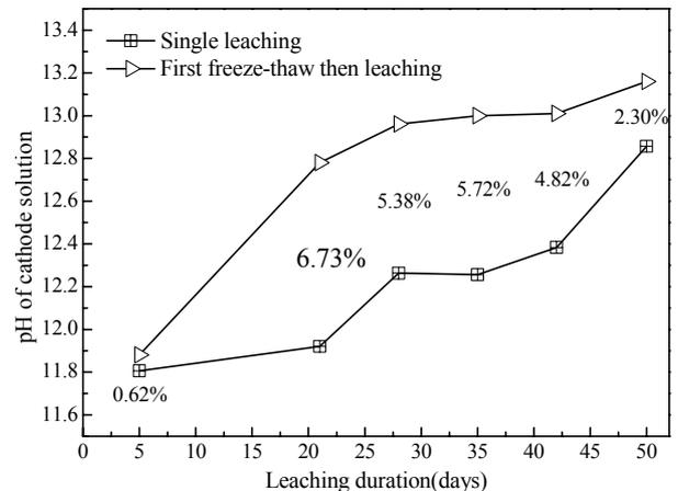
Fig. 3 - Comparison of pH variation in cathode room between single test and coupled test.
