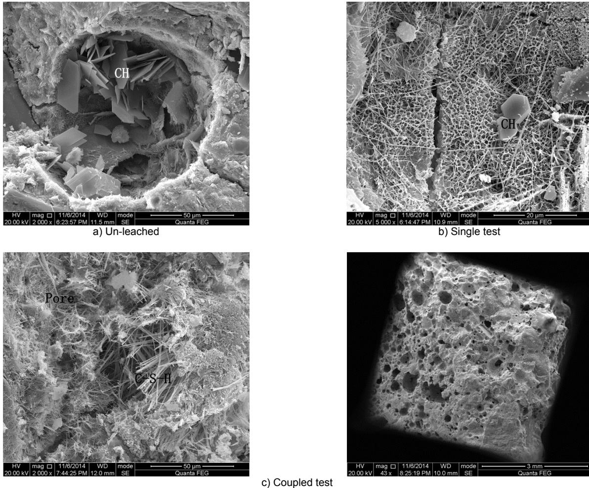
Fig. 5 - SEM images of a) un-leached specimen, b) single test and c) coupled .
