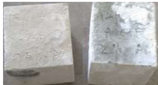
Fig. 11 - Specimens after exposed to acid and sulphate curing.
