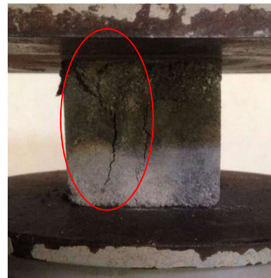
Fig. 10 - Failure pattern of AC10F2 specimen.
