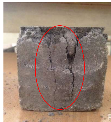
Fig.9 - Failure pattern of CC specimen.
