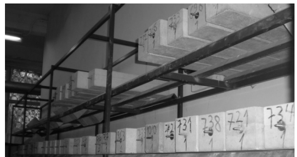
Fig. 4 – Concrete prisms for determination of the axial shrinkage.
