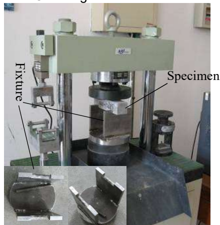
Fig. 3 - Loading devices for bending experiment.
