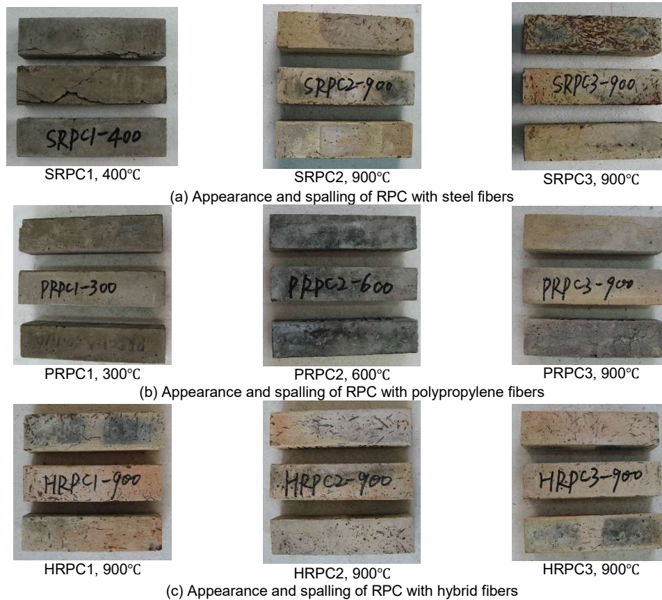
Fig. 4 - Change of RPC spalling with different fiber types and exposure temperatures.
