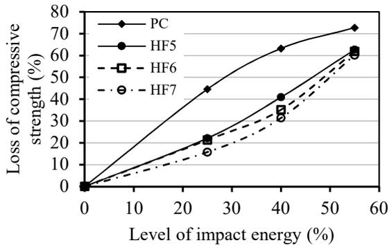
Fig. 2 - Loss of compressive strength versus level of impact energy for the hooked end steel FRC.
