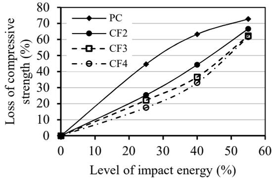
Fig. 1 - Loss of compressive strength versus level of impact energy for the crimped steel FRC.
