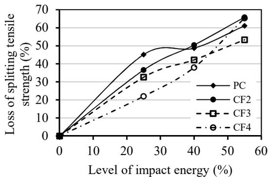
Fig. 3 - Loss of splitting tensile strength versus level of impact energy for the crimped steel FRC.
