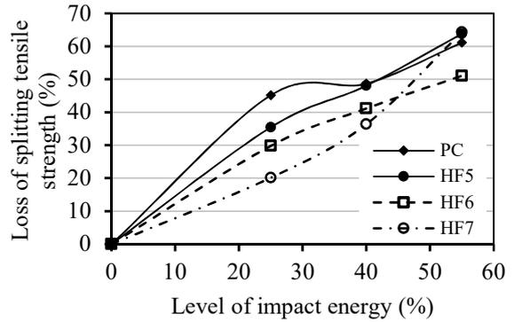
Fig. 4 - Loss of splitting tensile strength versus level of impact energy for the hooked end steel FRC.
