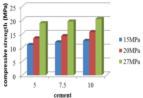
Fig.4 - Compressive strengths of PG-CS-HL-PC full bricks versus cement content and compaction pressure (phosphogypsum=70%).
