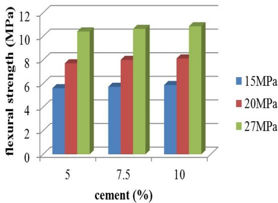
Fig.6 - Flexural strength of PG-CS-HL-PC full bricks versus cement content and compaction pressure (phosphogypsum=60%) .
