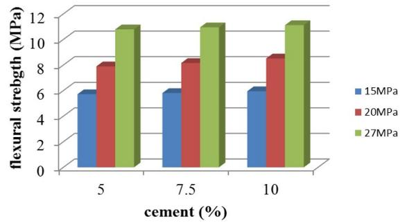
Fig.7 - Flexural strength of PG-CS-HL-PC full bricks versus cement content and compaction pressure (phosphogypsum=70%) .
