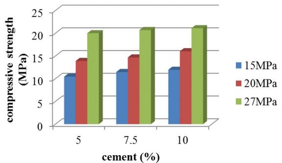
Fig.5 - Compressive strengths of PG-CS-HL-PC full bricks versus cement content and compaction pressure (phosphogypsum=80%).
