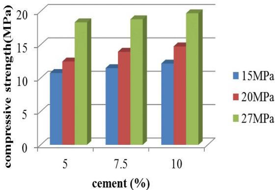
Fig.3 - Compressive strengths of PG-CS-HL-PC full bricks versus cement content and compaction pressure (phosphogypsum=60%).
