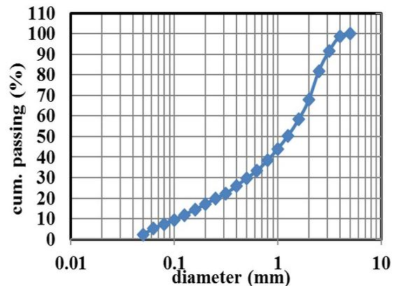
Fig. 2 - Granulometric curve of the crushing sand.
