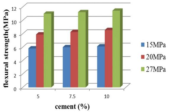
Fig.8 - Flexural strength of PG-CS-HL-PC full bricks versus cement content and compaction pressure (phosphogypsum=80%) .
