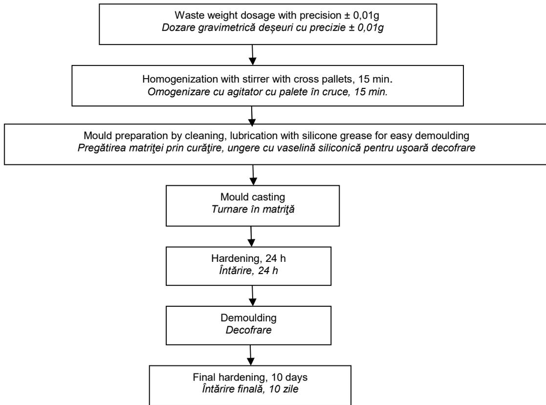
Fig.2 – Schema of the technological process for obtaining the oxide materials / Schema procedurii tehnologice de obținere a materialelor oxidice.
