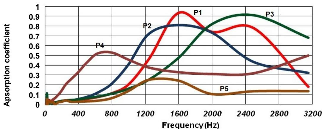
Fig. 4 - Sound absorption coefficient versus the sound wave frequency, for the obtained oxide materials / Coeficientul de absorbtie a undelor sonore in functie de frecventa undelor sonore, pentru materiale oxidice elaborate.
