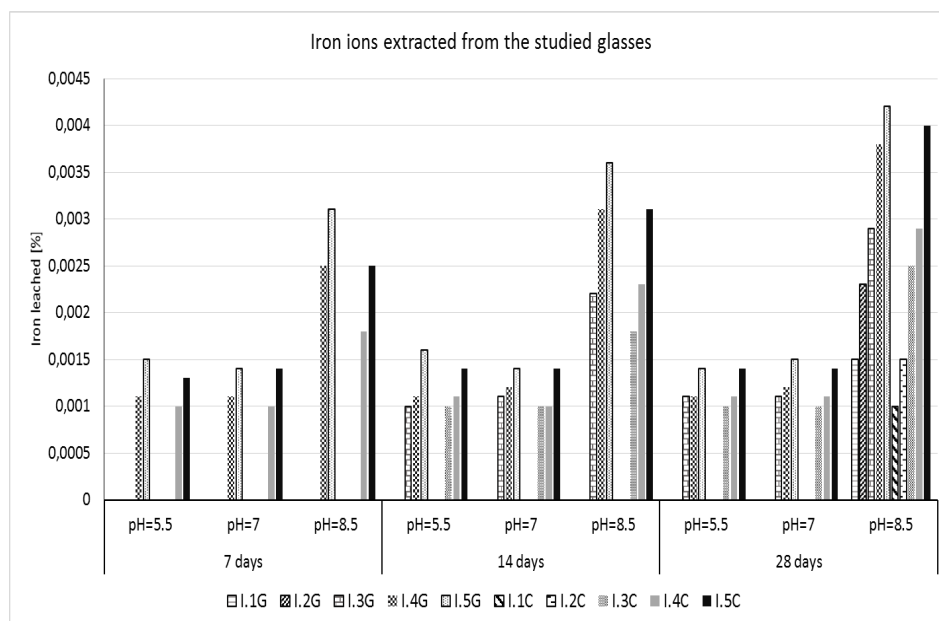
Fig.5 - Iron ions losses from the studied glasses / Pierderile de ioni de fier din probele studiate.
