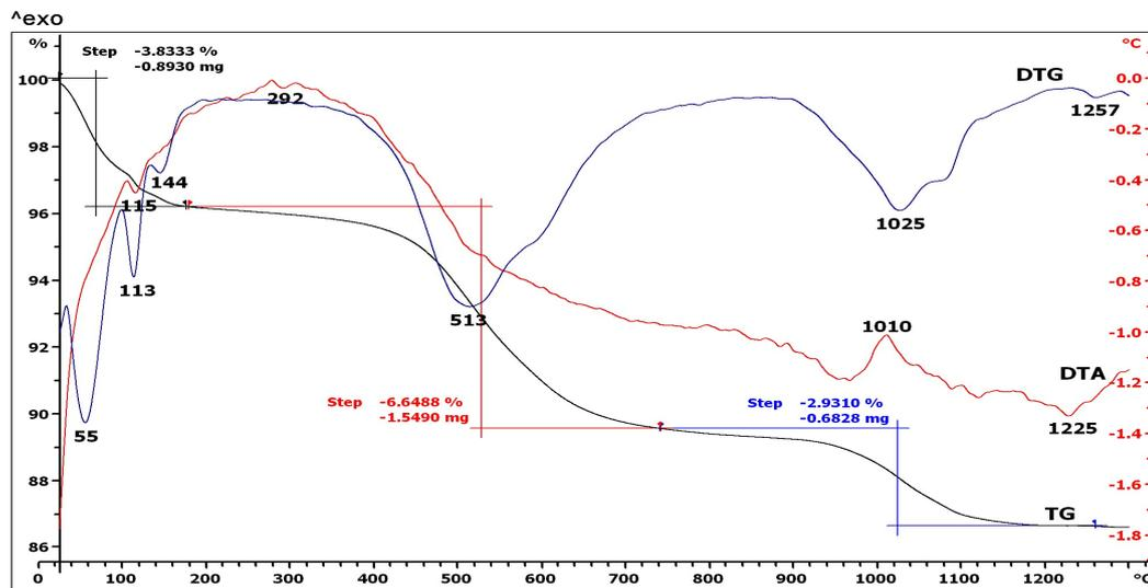
Fig. 2b - TG/DTA diagram for clay / Diagrama TG / DTA a argilei.
