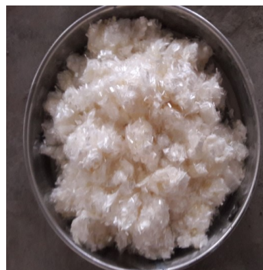
Fig 2 - Typical view of PVA fibers.
