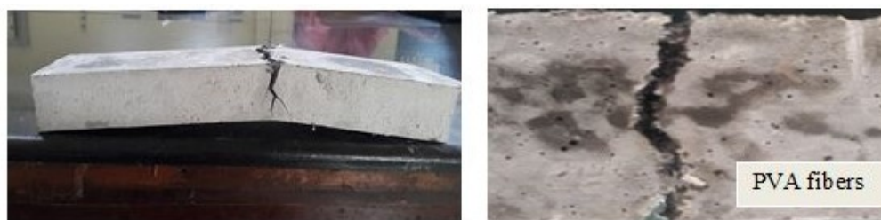
Fig 10 - Failure patterns of ECC prisms.
