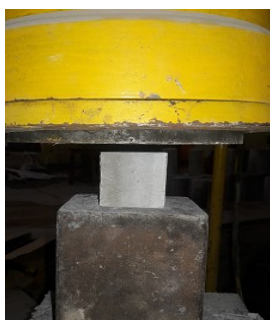
Fig 4 - Typical view of compressive strength test set up.
