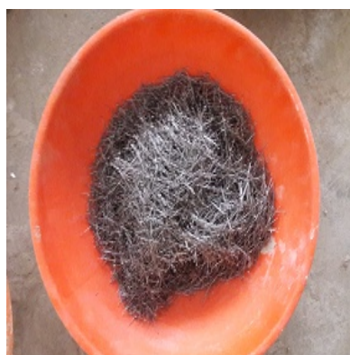
Fig 1 - Typical view of hooked-end steel fibers.
