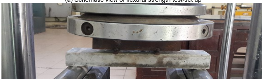
(b) Typical view of flexural strength test-set up
