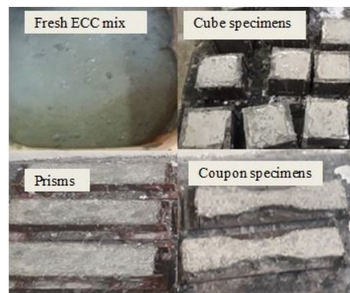
(a) Fresh ECC mortar mix (b)
