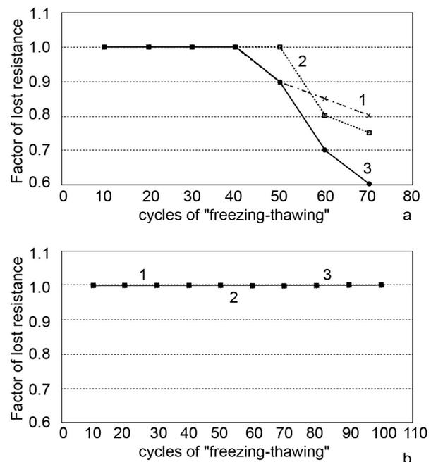
Fig. 1. - Freeze-thaw resistance of the glued materials (No 5, Table 2)(a - without filler/ additive; b - with filler/ additive): 1 - “concrete-concrete”, 2 - “concrete-ceramics”, 3 - “ceramics-ceramics”
