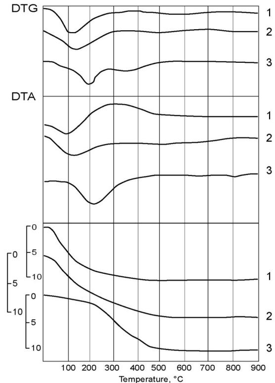
Fig. 3 - DTA-curves of hydration products of the geocement-based adhesives (No 2, Table 2): 1 – after hardening at  $t = 20^\circ C$ ; 2 – after hardening for 12 months at  $t = 20^\circ C$ ; 3 – after 10-times autoclave treatment (pressure = 8 atm).
