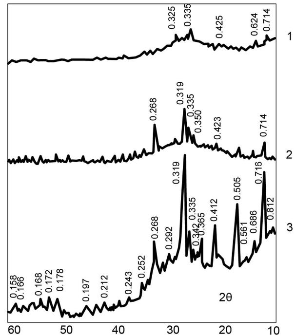
Fig. 2 - X-ray spectra of hydration products of the geocement-based adhesives: 1 – after hardening at  $t = 20^\circ C$ ; 2 – after hardening for 12 months at  $t = 20^\circ C$ ; 3 – after 10-times autoclave treatment (pressure = 8 atm).
