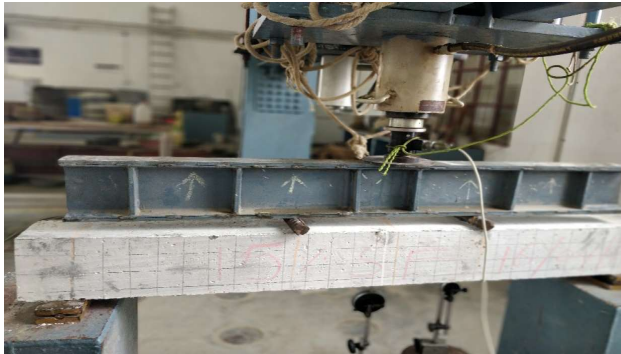
Fig 3 -Testing of Beam Specimen.
