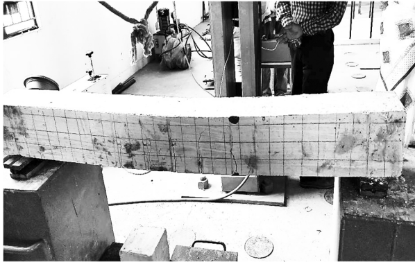
Fig. 6 -Beam – Failure by Bending
