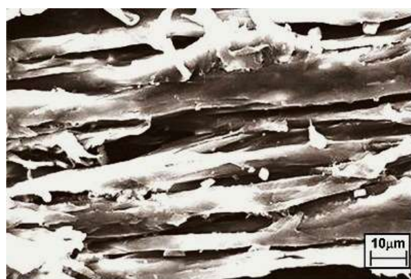
Fig 2 (e) - SEM Image of the composites of 8wt% nanoclay.
