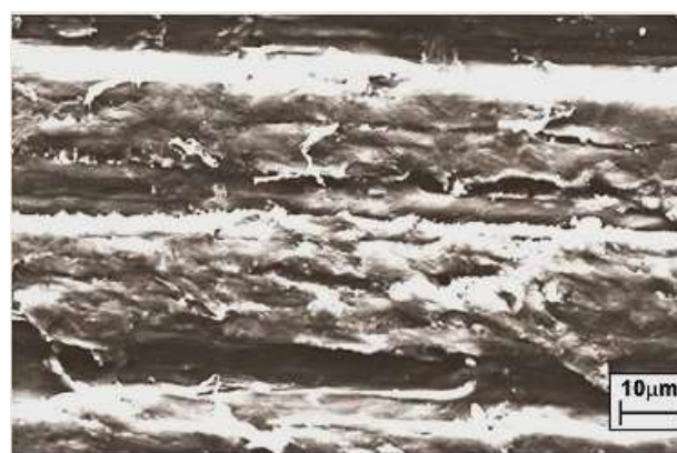
Fig 2 (f) - SEM Image of the composites of 10wt% nanoclay.
