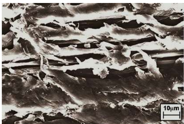
Fig 2 (c) - SEM Image of the composites of 4wt% nanoclay.
