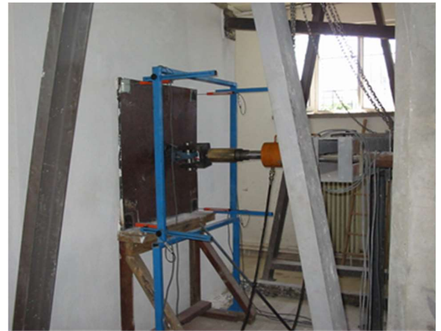
Fig. 5 – Placement of measuring devices on the wall.
