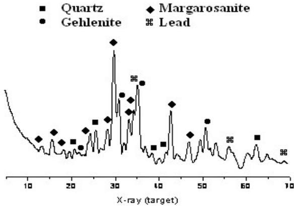
Fig. 1 - X-ray diffraction of lead slag / Difrakția de raze X a zgurii de plumb.
