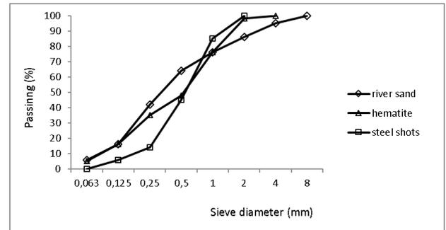
Fig. 2 - Grading curve of the some aggregate/Curba de granulozitate a unor agregate.
