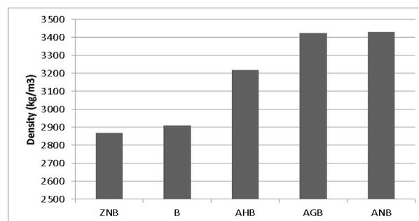
Fig. 3 - The apparent density of the concretes with various aggregate types/ Densitatea aparentă a betoanelor cu agregate diferite.
