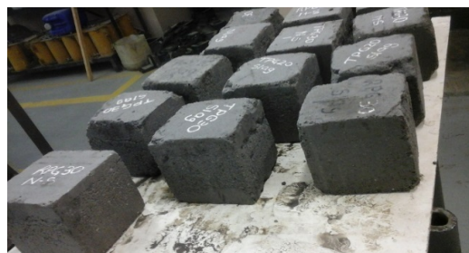
Fig.1 - Images of RPG and TPG cured at 80°C for 96 hours.
