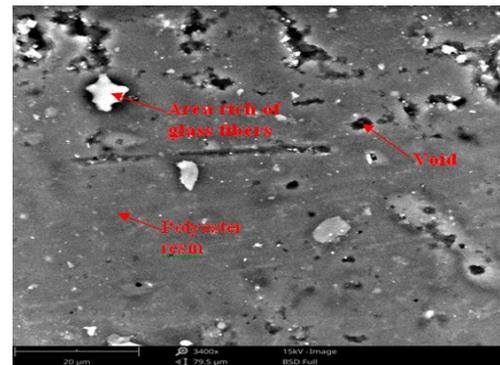
Fig. 2 - A surface SEM view with one of the samples *O vedere SEM a suprafeței unei epruvete .*
